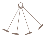
4 pegs combined in one anchoring point
