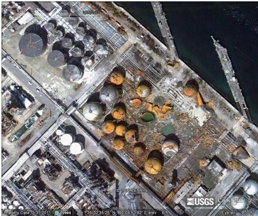
FIGURE 2.5 The Refinery's LPG Tank Farm After the Fires and Explosions Triggered by the Tohoku Earthquake
