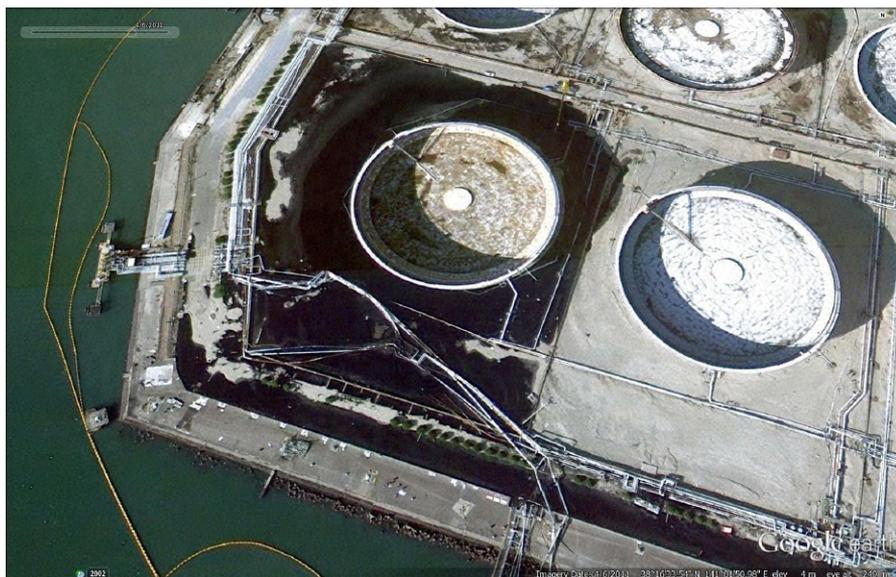
FIGURE 2.7 Hydrocarbon Releases From Damaged Pipelines at Sendai Refinery due to Tsunami Impact
