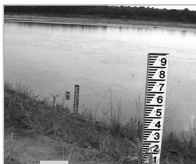
Figure 4.3: Water level-gauge installed at the river bank
