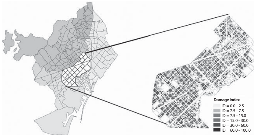
Figure 3.4 Barcelona Physical Seismic Risk
