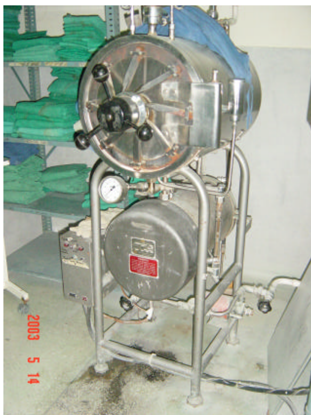
Photo 11: Autoclave machine needs anchorage at the base.
