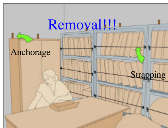
Fig 1: Life safety hazards can be reduced just by removing less important things from the working place.
