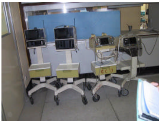
Photo 8: ECG monitors on rollers with potential risk of sliding and overturning.
