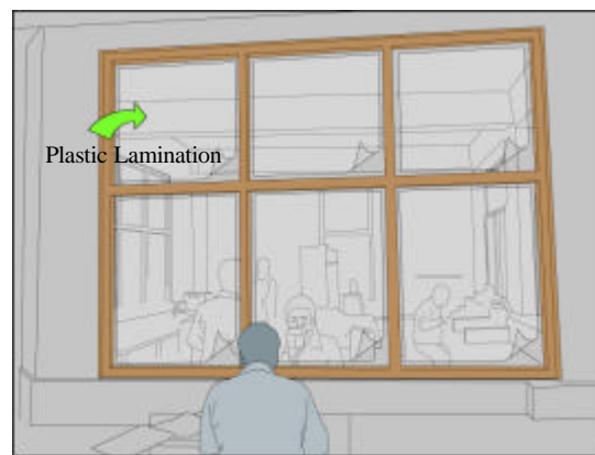
Fig 12: Simple plastic lamination can protect lives.
