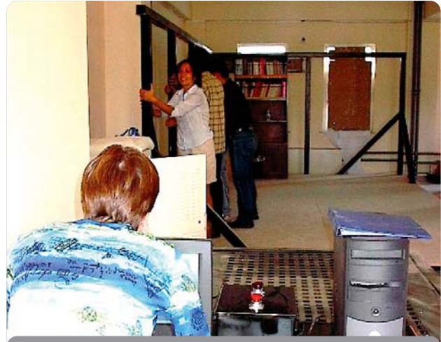
Bogazici University researchers use a shake table to simulate an earthquake and to identify best practices for NSM.
