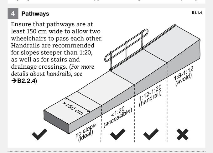
Compacted gravel or selfbinding aggregate is suitable as ground cover for pathways. Provide shaded resting places at 100-200 metre intervals along main circulation routes.
