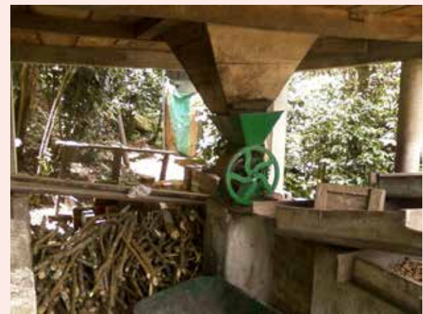
A coffee de-pulper, which is an important component of wet processing. (Photo: Nicaraguan Red Cross)
