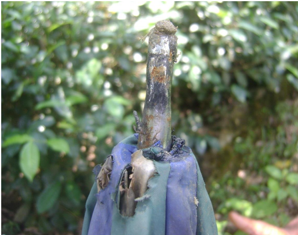
Figure 3. Path to ground through an umbrella hung on the shelter.
