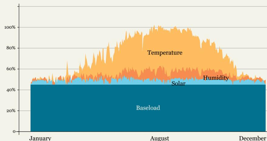
Figure 16 Contribution of cooling to electricity load in Abu Dhabi throughout the year.<sup>135</sup>
