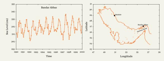
Figure 4 Sea level at Bandar Abbas between 1990 – 1999 (left) and location of Bandar Abbas tide gauge (right).
