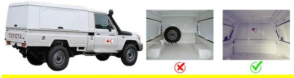
Warning: Do not keep the spare wheel inside the cargo space to avoid contamination during tyre replacement.
