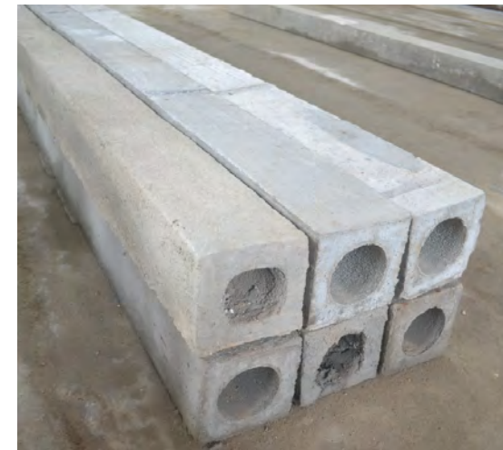
Ferrocement Hollow Column
