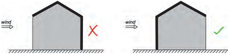
Shelter with an open facade - wrong and right
