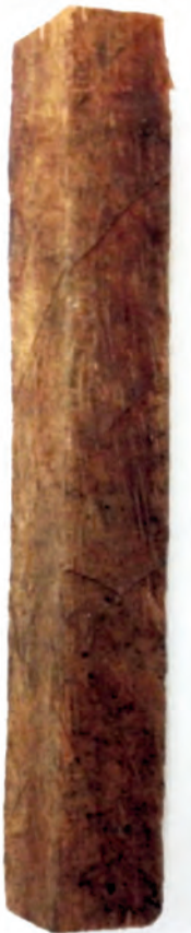
Coconut wood cut from sapwood (high density) (IFRC-SRU)
