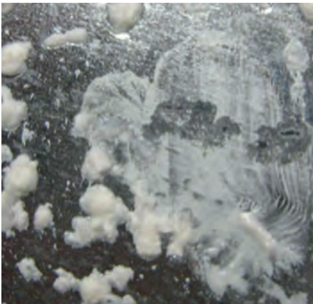
Sheets with heavy wet storage stain should be rejected
