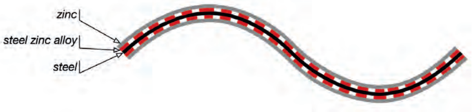
Chapter of CGI sheet showing the layers of coating
