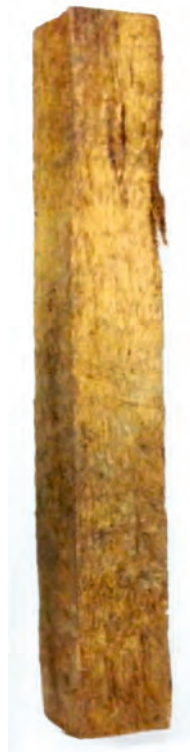
Coconut wood cut from heartwood (medium to low density) (IFRC-SRU)
