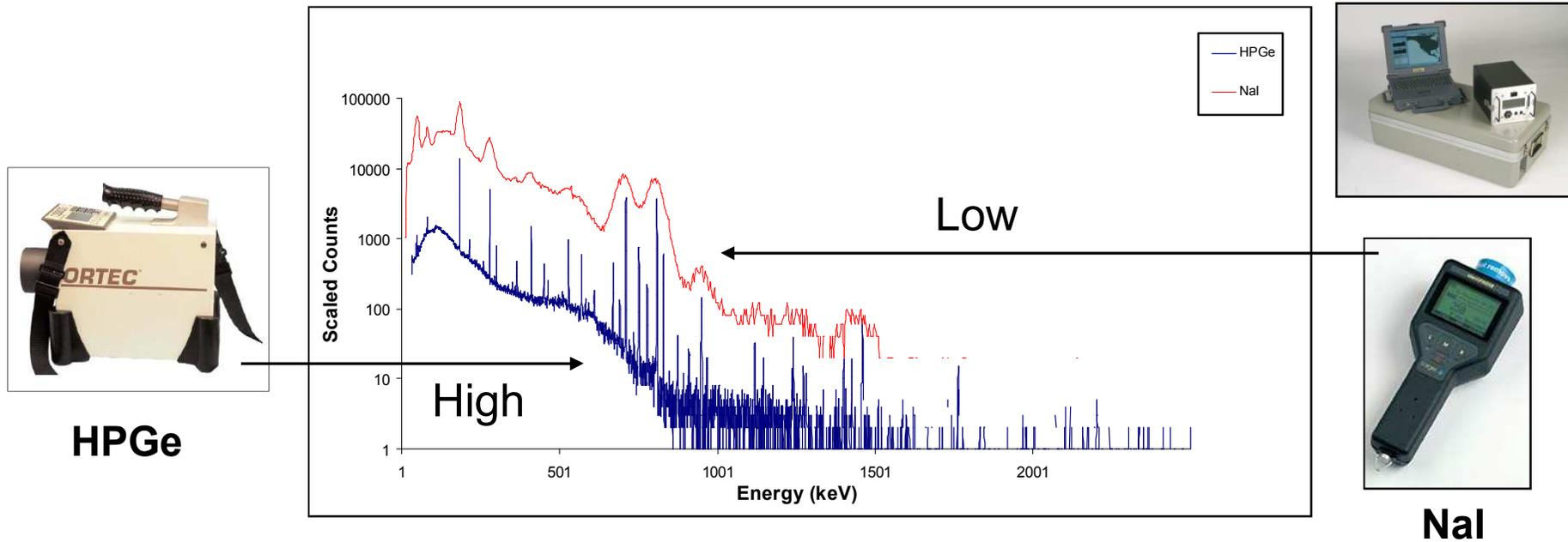
*Comparison of a sodium iodide spectrum (low resolution) to a high purity germanium spectrum (high resolution)*
