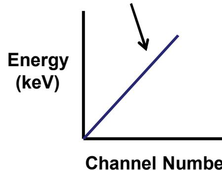
The energies are used to calibrate the energy scale using a linear relationship ( $y=mx+b$ )
