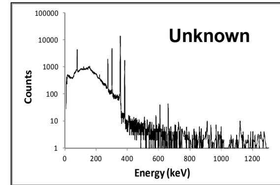
An unknown spectrum is then measured and the radioisotope identified by the gamma-ray energies
