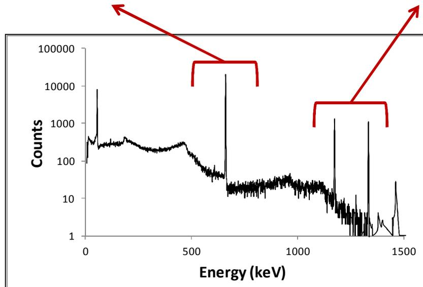
Gamma-ray peaks have Gaussian shapes. The centroid is the gamma-ray energy and the area under the peak is proportional to the radioactivity of the source.
