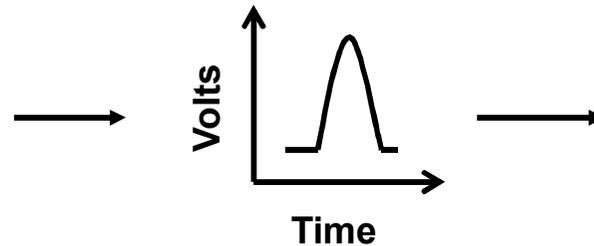
The detector electronics converts the energy to an electronic pulse with 0-8 volts
