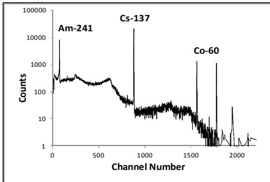
A spectrum of known radioisotopes and gamma-ray energies is measured
