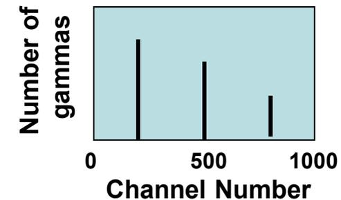
A multi-channel analyzer bins the voltages of the electronic pulses into channels
