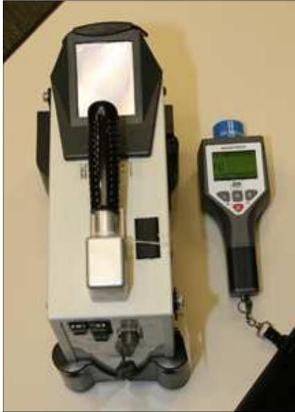
If a RIID is too close to the Detective during a measurement, then the Cs-137 calibration source in the RIID can be detected
