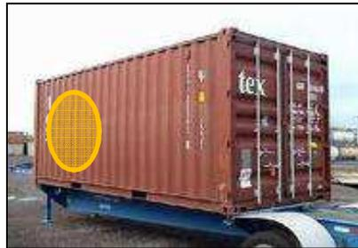
A vehicle or cargo container with a point source may appear as a *localized source* in dose rate measurements
