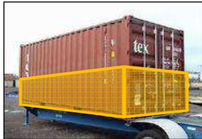
A vehicle or cargo container filled with NORM may appear as a *uniformly distributed* source with nearly equal dose rates on all sides
