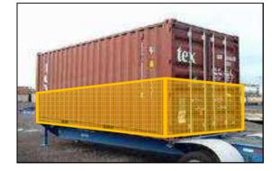
A vehicle or cargo container filled with NORM may appear as a *uniformly distributed* source with nearly equal dose rates on all sides.
