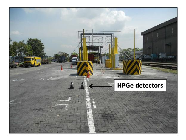
In order to acquire background measurements, the Detective HPGe detectors were placed about 50 meters from the cargo containers.
