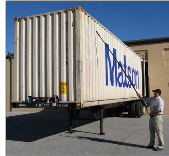
A tele-probe can be used to map a container which is on a trailer
