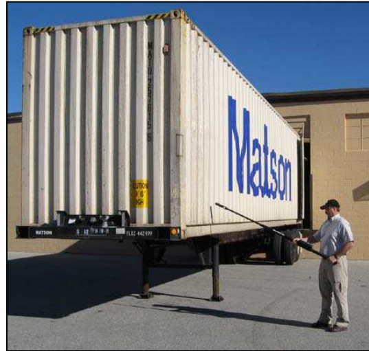
A tele-probe can be used to map a container which is on a trailer
