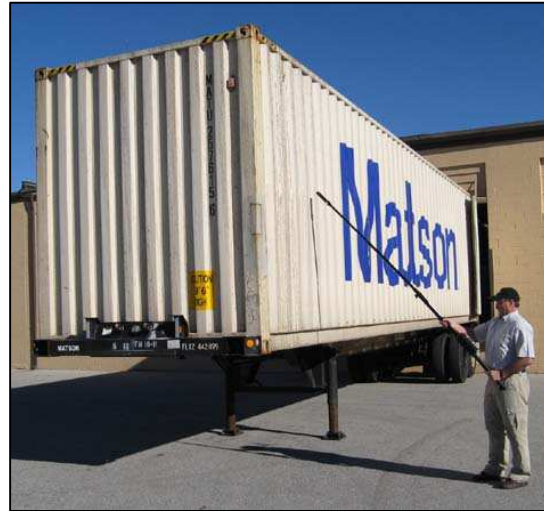
A tele-probe can be used to map a container which is on a trailer
