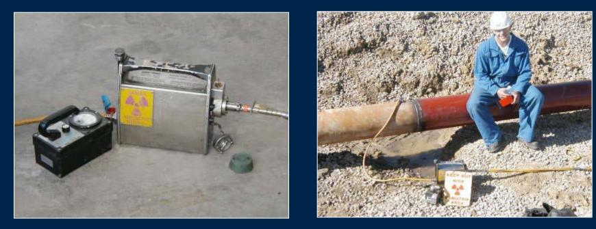
High activity <sup>192</sup>Ir sources are typically used to radiograph welds in pipes.
