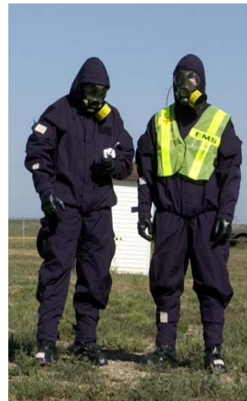
Figure 6 Two-piece CBRN Personal Protective Equipment with C4 Respirator and FR64 NIOSH-Approved Canister
