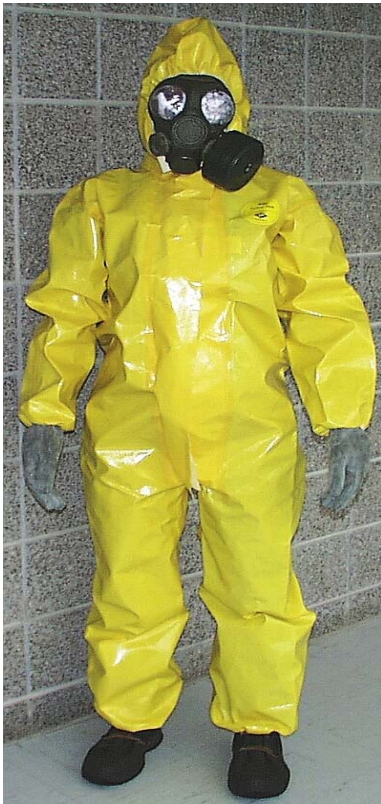
Figure 3 Level “C” PPE with C4 Respirator and FR64 Canister
