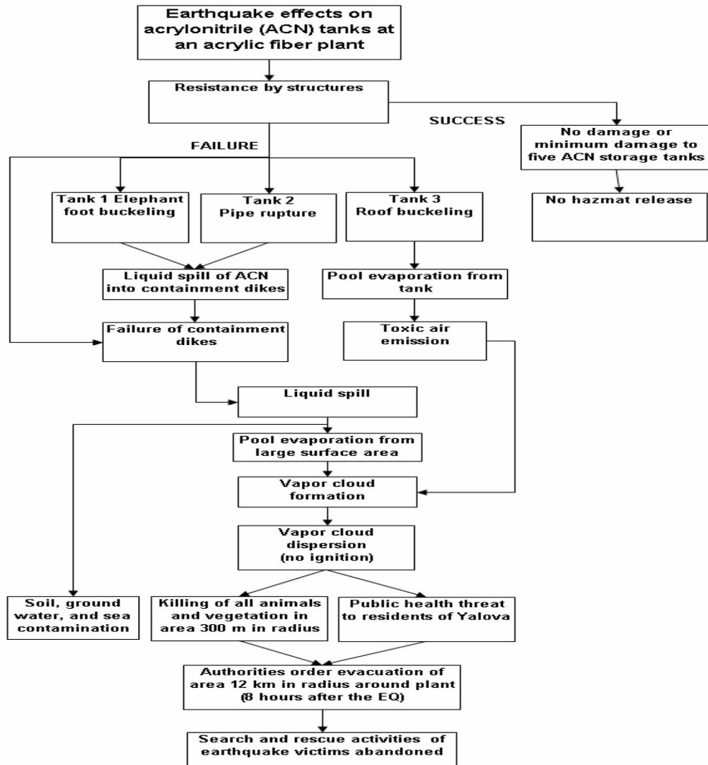
Figure A2.e - Earthquake effects on acrylonitrile storage tanks at the acrylic fibre plant.
