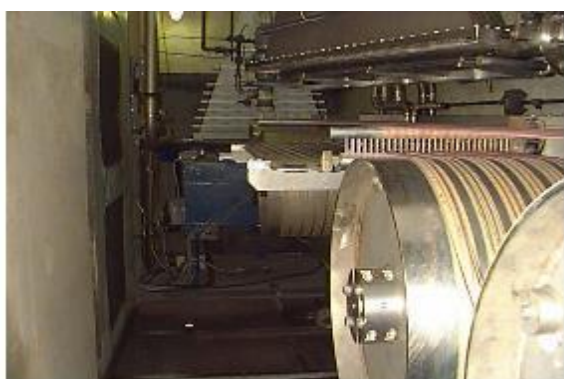
a) Electron Beam Accelerator JOB 307 (Dynamitron®) energy 1.5 MeV, beam current 65mA, scan 60 to 120 cm, beam power 97.5 kW
