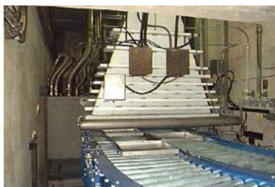
b) Electron Beam Accelerator JOB 188 (Dynamitron®) energy 1.5 MeV, beam current 25mA, scan 60 to 120 cm, beam power 37.5 kW.
