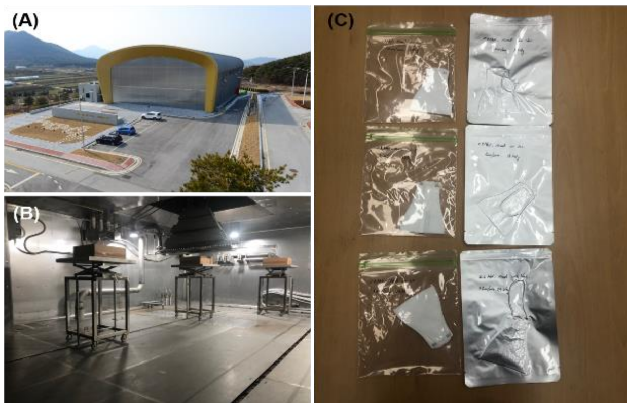
FIG. 1.2 (A)Electron Beam Demonstration and Research Building (B)2.5MeV electron beam accelerator(Model: ELV-8, Manufacturer: EB-Tech, Korea) (C)Samples before electron beam and gamma irradiation under air(left) and vacuum(right) condition
