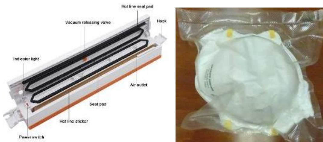
FIG. 5. Household vacuum sealer (left). Sealed vacuum bag mask sample G after irradiation (right).
