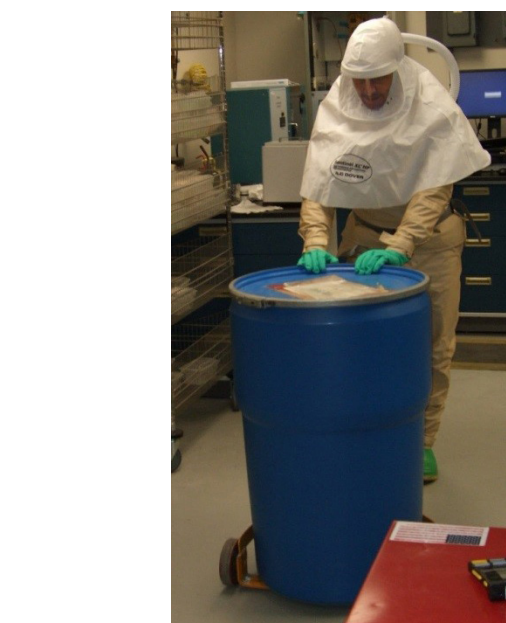
EXHIBIT 11 Ensemble Being Evaluated for Overall Function by Test Subject Moving 55-Gallon Drum. (Courtesy of Intertek Testing Services.)
