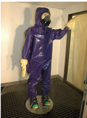
EXHIBIT 7 Ensemble Being Evaluated for Overall Liquid Integrity. (Courtesy of International Personnel Protection, Inc.)
