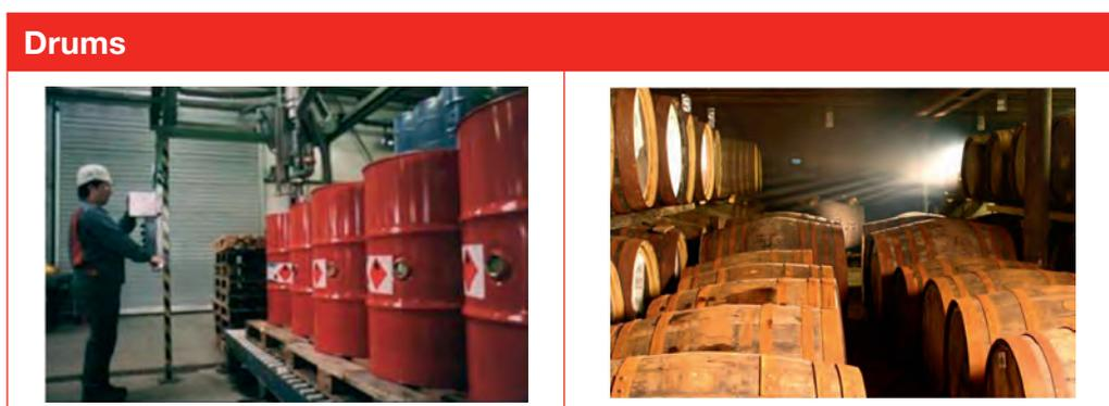
**7C3.211** One example of where non-UN approved packaging is used to transport dangerous goods is the use of oak barrels to transport alcoholic beverages such as Scotch whisky.
