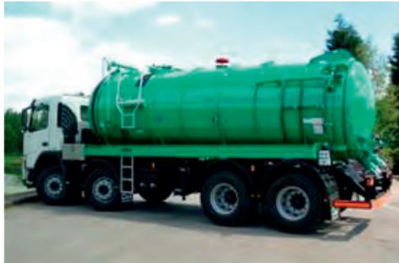
**7C3.202** The photo above shows a vacuum-operated tank; notice should be taken of the external strengthening ribs which are to prevent the tank collapsing when the vacuum is applied. Details of the specifications regarding vacuum operated waste tanks can be found in Chapter 6.10 of ADR Volume II.
