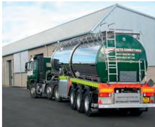
**7C3.201** The photo above shows a 30,000 litre non-pressure, stainless steel, multi-compartment tanker that can carry a variety of substances at different times but only compatible loads during any single journey.
