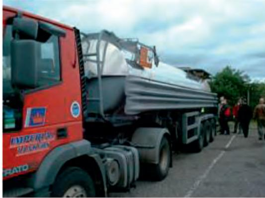
**7C3.200** The photo above shows a non-pressure tank containing Nitric Acid >70 per cent. Note the added protection to prevent accidental damage to the structure of the tank, which is a good indication that the tanker carries a high consequence load.
