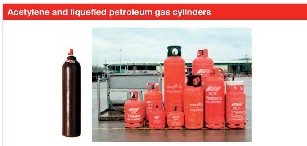
**7C5.50** To distinguish positively between acetylene and other non-liquefied petroleum gas cylinders is more difficult when they have been subjected to a fire.
