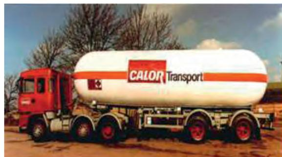
**7C3.203** The above photo shows a typical pressure tank designed for carrying liquid petroleum gas.
