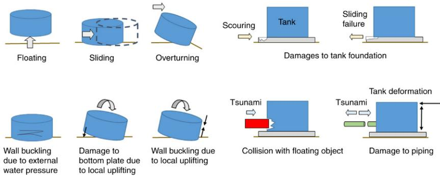
FIGURE 13.4 Failure Modes Observed During the Great East Japan Tsunami in 2011
