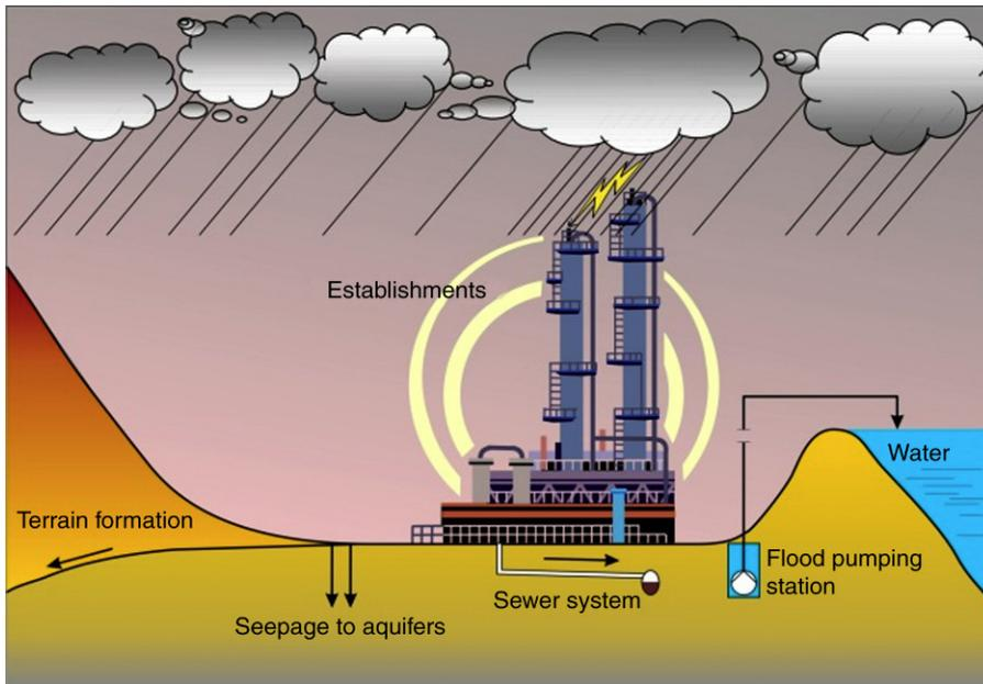
FIGURE 8.7 Potential Water Runoff Routes From a Site
