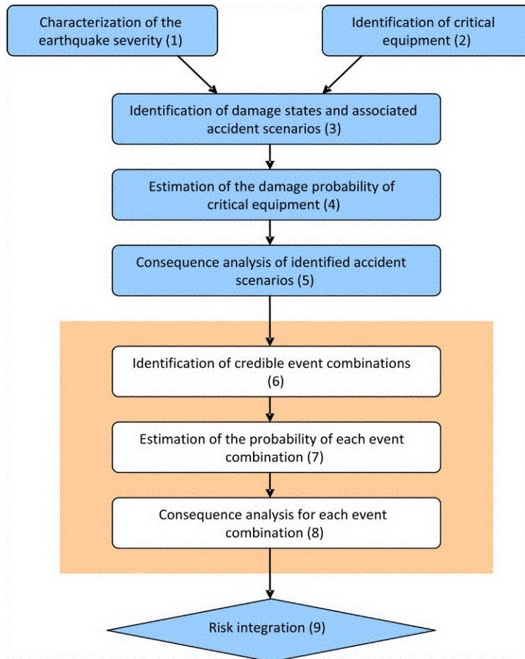
FIGURE 7.3 Flowchart Showing the Procedure for Seismic Natech Risk Analysis
