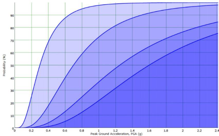
FIGURE 8.2 Fragility Curve for an Anchored Steel Storage Tank Subjected to Earthquake Shaking
