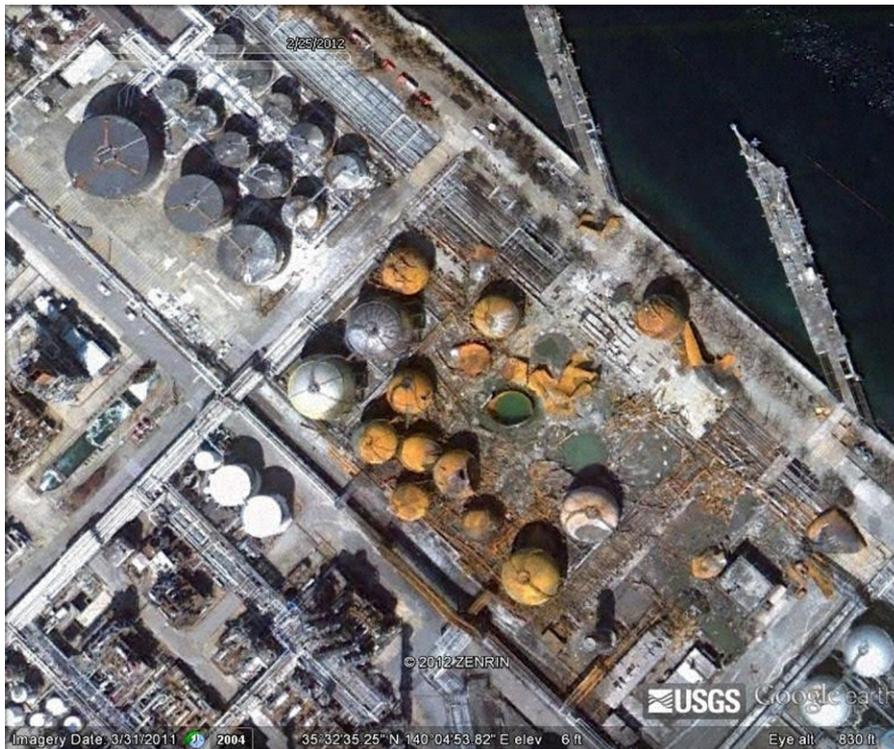
FIGURE 2.5 The Refinery's LPG Tank Farm After the Fires and Explosions Triggered by the Tohoku Earthquake
