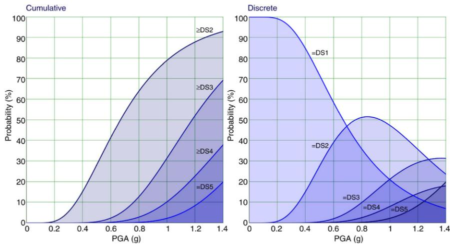
FIGURE 10.4 Example Cumulative and Discrete Fragility Curves [O'Rourke and So (2000),  $H/D < 0.7$ ]
