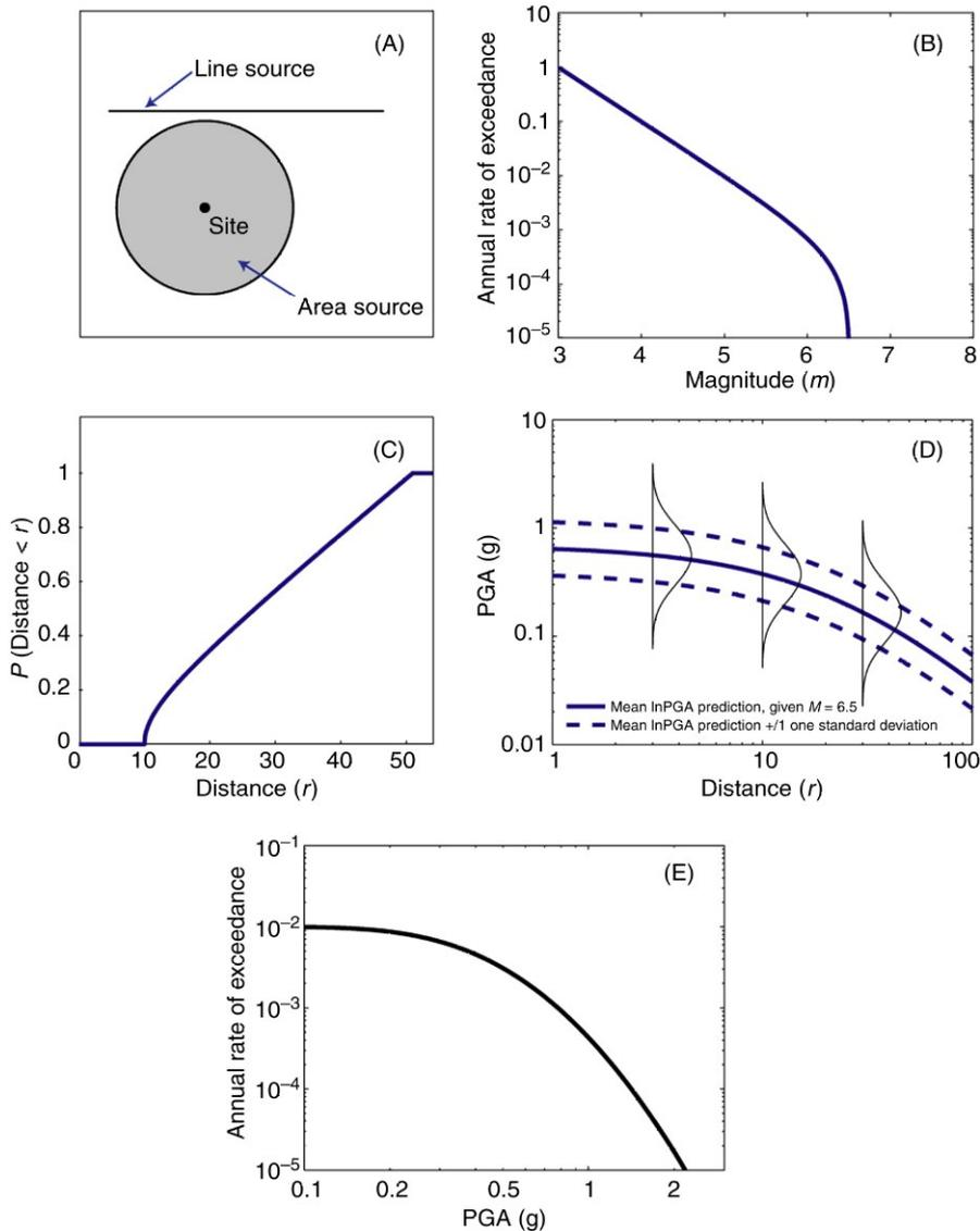
FIGURE 5.1 Schematic of the Five Basic Steps in Probabilistic Seismic Hazard Analysis According to Baker (2008)
