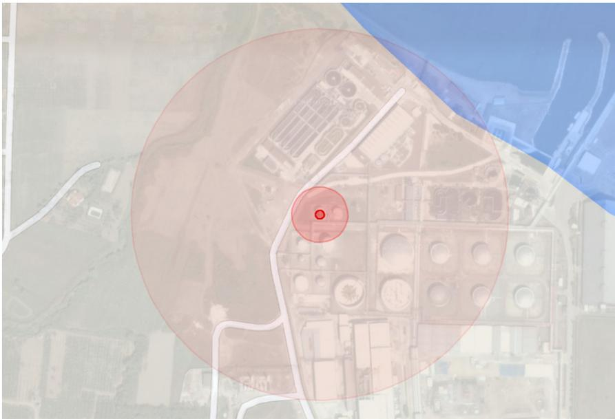
**FIGURE 10.5 Natech Impact Zone for Heat Radiation From Tank T-1 Containing Methanol (Base Image ©2016 DigitalGlobe)**
