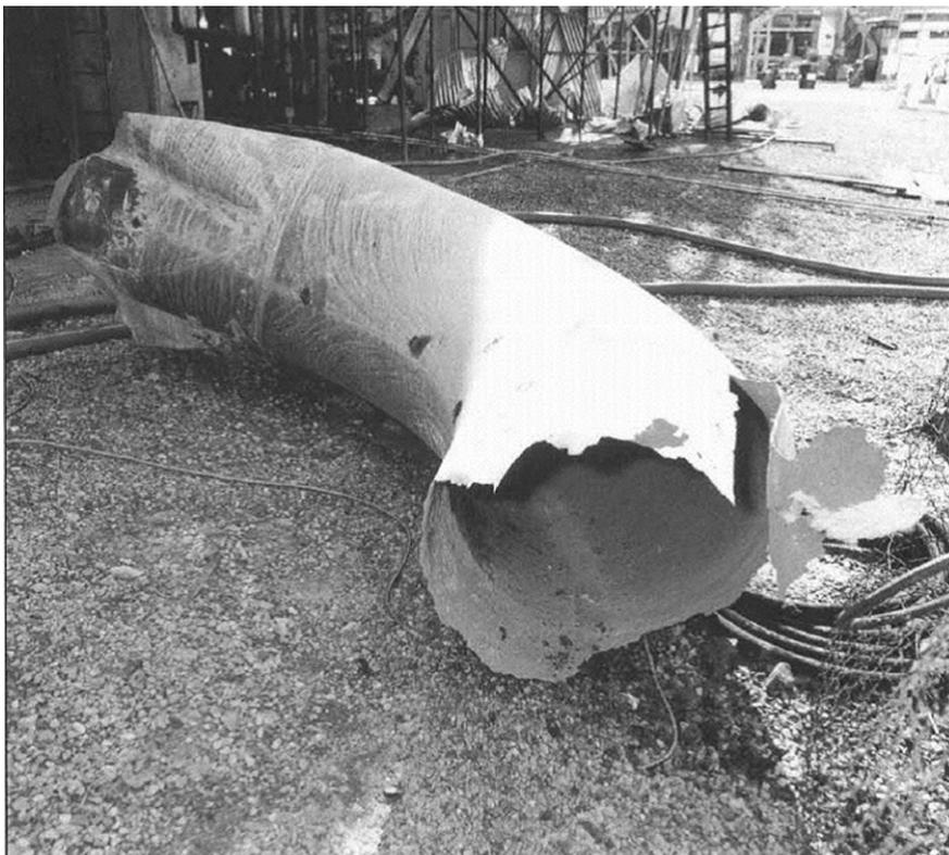
FIGURE 2.9 The Failed Elbow Bend at the 30-in. Flare Drum Outline Line From Which the Hydrocarbons Were Released
