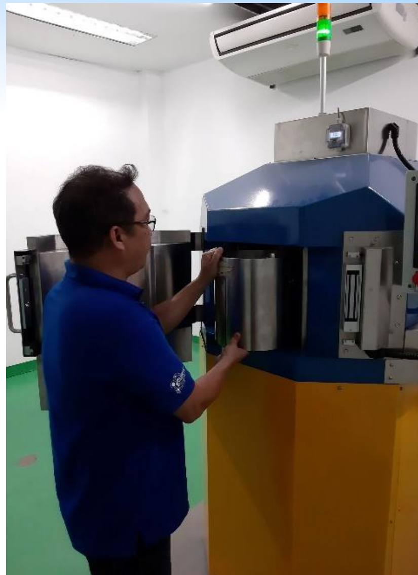
Operator loading the samples in the Ob-Servo Sanguis Gamma Irradiator
