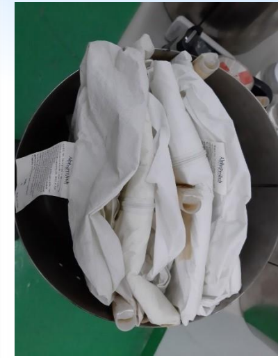
Arrangement of PPE as irradiated at the Ob-Servo Sanguis Irradiator (top view)
