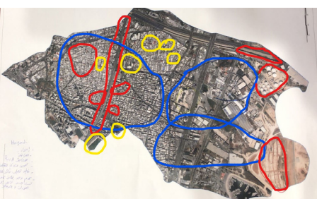
Photo: Using A1 printed maps to identify hazards (red), capacities (yellow), exposure (blue) by hand as polygons. This will later be translated into fully digital maps.
