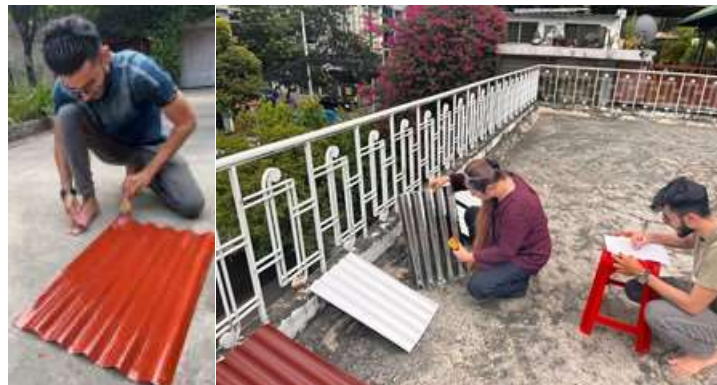
Figure 3: Action research program was undertaken that looked at passive heat resistant solution using locally available iron oxide rust proof coating paint.
