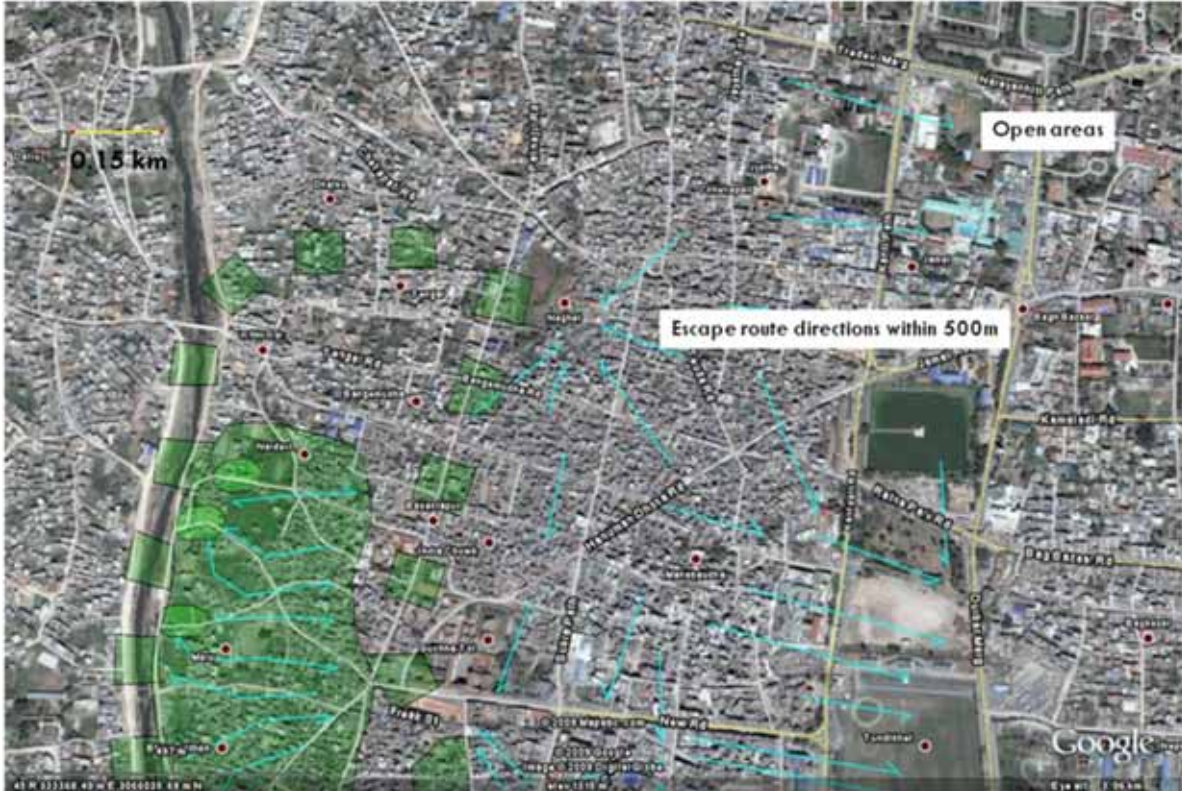
Figure 5.17 Escape Route Planning North of Core
