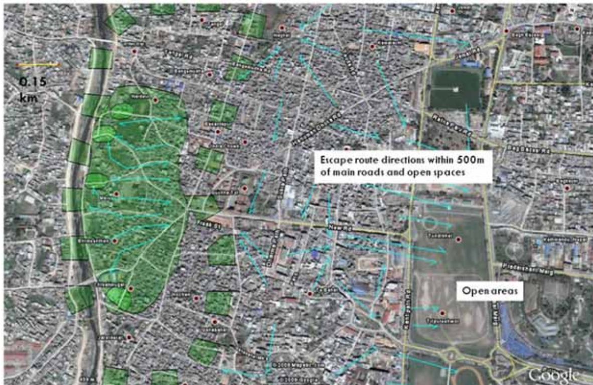
Figure 5.18 Escape Route Planning Around Core
