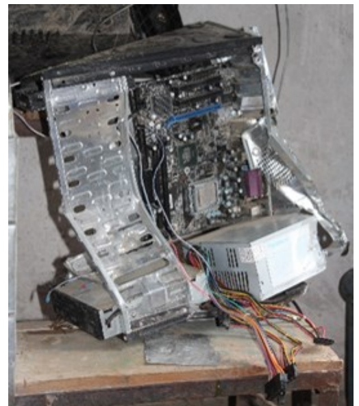
Figure 11. School computers and lab supplies were damaged where no non-structural mitigation measures had been taken. Photo: R. Paci-Green/Risk RED
