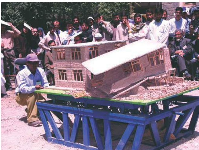
Models of traditional structures with and without hazard-resistant construction show remarkably different behaviour when shaken on a simple shake table during a community demonstration in Kabul, Afghanistan. Photo: Bishnu Pandey.
