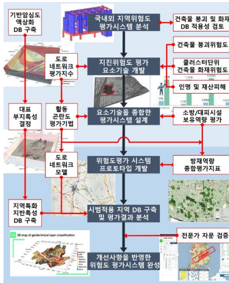
Figure 4: Earthquake Risk Assessment Technology
