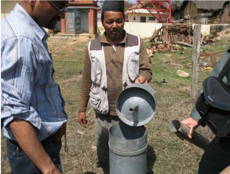
Figure 2.25 Non-recording bucket type rain gauge at Jalkundi (Station 360, DHM)
