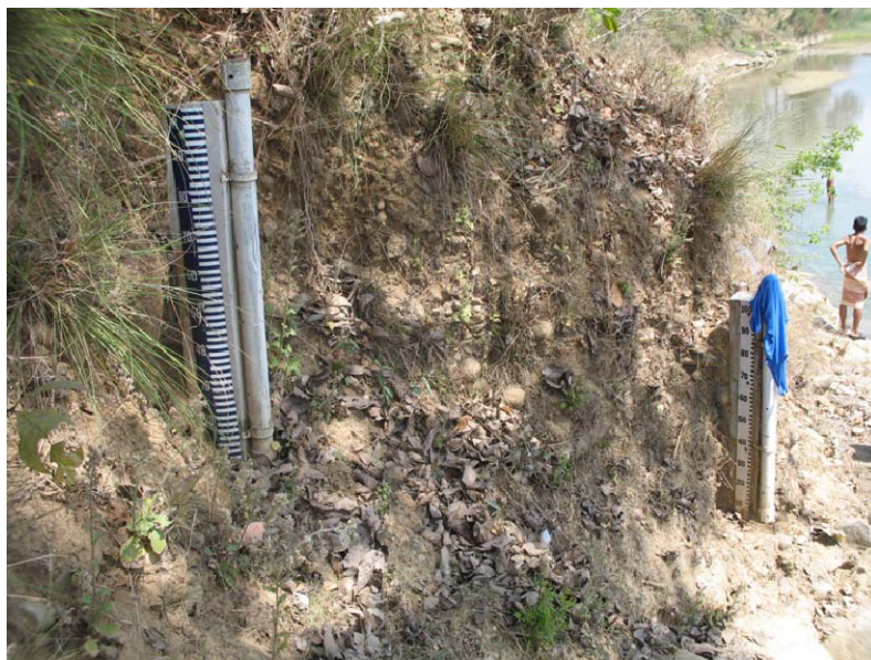
Figure 2.26 Water Level gauge staffs at Jalkundi (Station 360) with simple device for recording instantaneous maximum flood
