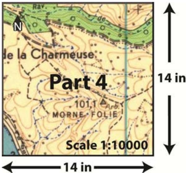
3. Divide the current scale (1:10,000) by the desired scale (1:1,000). The result is 10.
