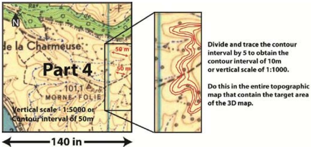
If the contour interval of the topographic map is originally 10m, then there is no need to go through the process of dividing and tracing new contour intervals.
