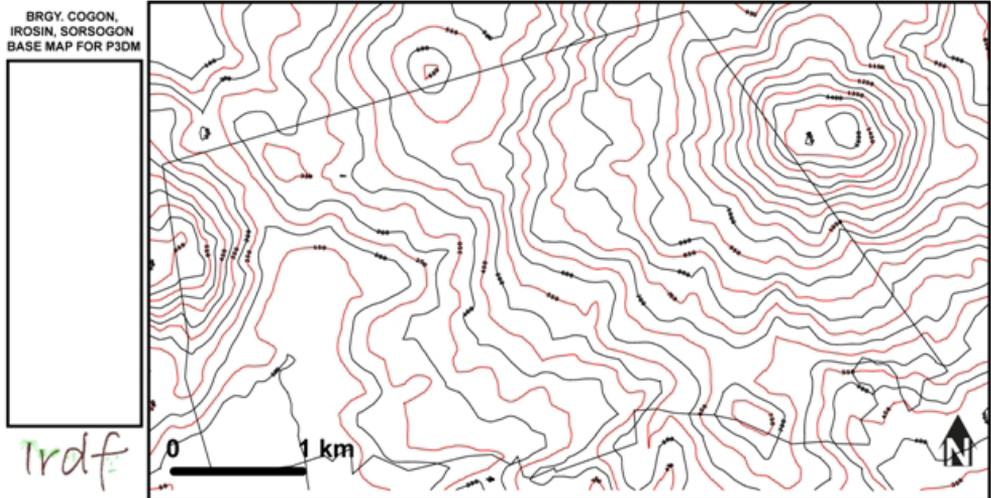
**Figure 6** – A sample of a base map with the basic elements required such as contours, scale and orientation (pointing to the north when relevant). Contours are portrayed using two different colors to better differentiate them.
