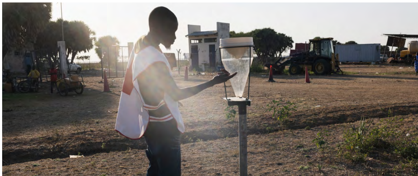
A Red Cross volunteer inspects a rain gauge used for local rainfall monitoring as part of a community early warning system in Chad. © Guillaume Binet / IFRC
