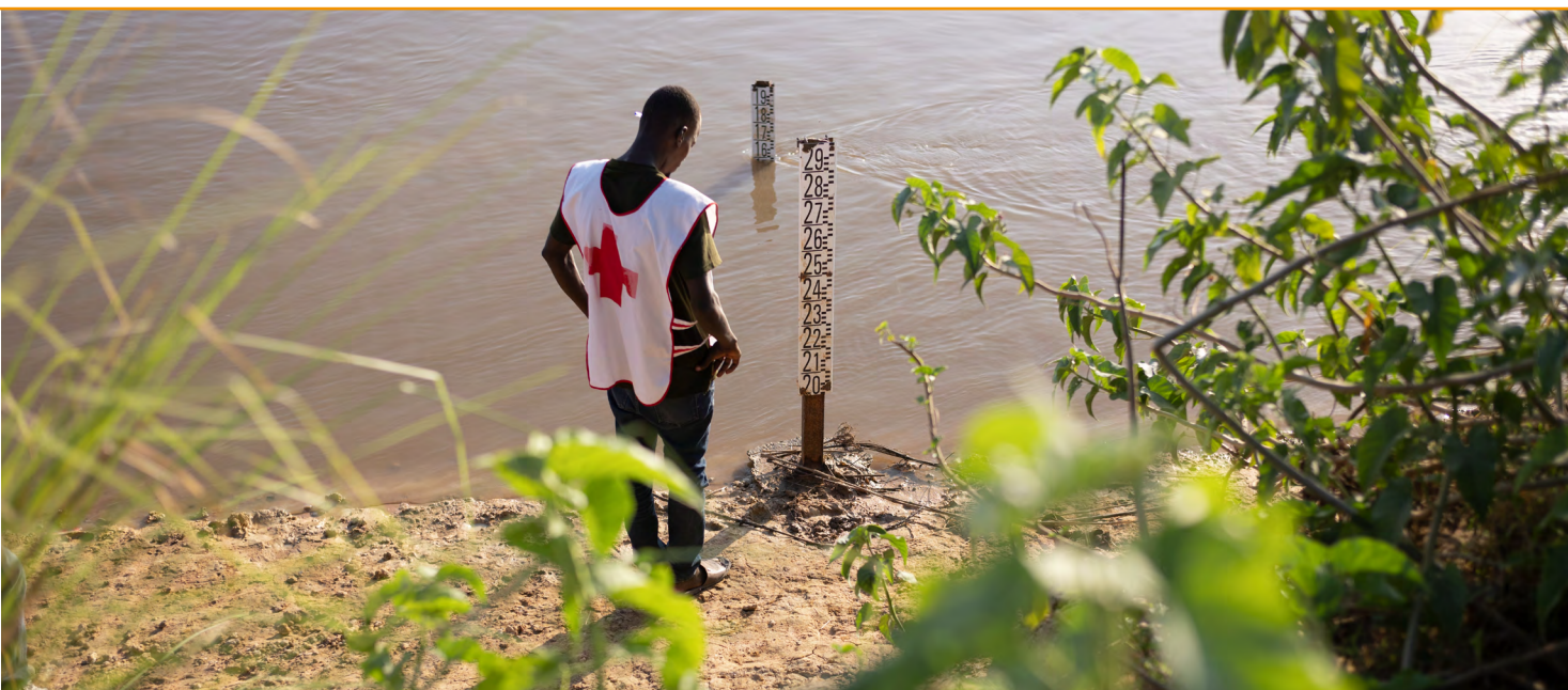
A Red Cross volunteer checks a river-level gauge during rain-gauge verification for a community early warning system in Djoumane, Chad. © Guillaume Binet / IFRC
